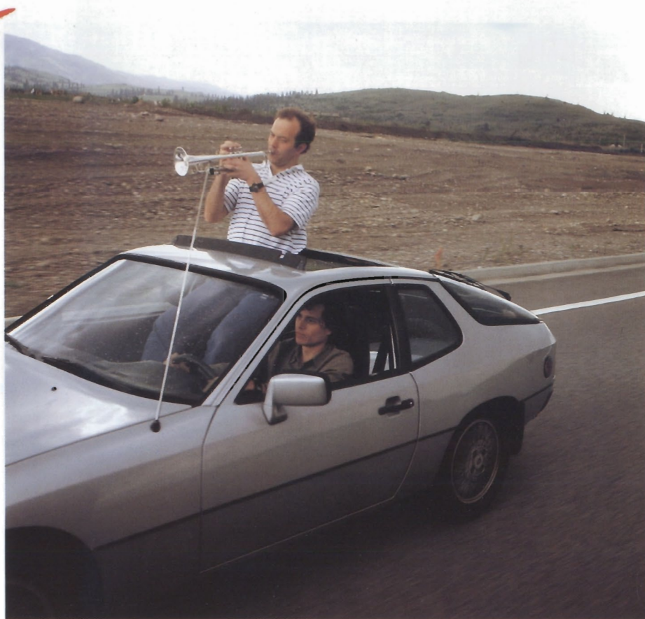
To explain the Doppler effect—a principle involving the frequency of sound waves—Mark drives down a long stretch of highway while Dave hits a high note on a trumpet.
